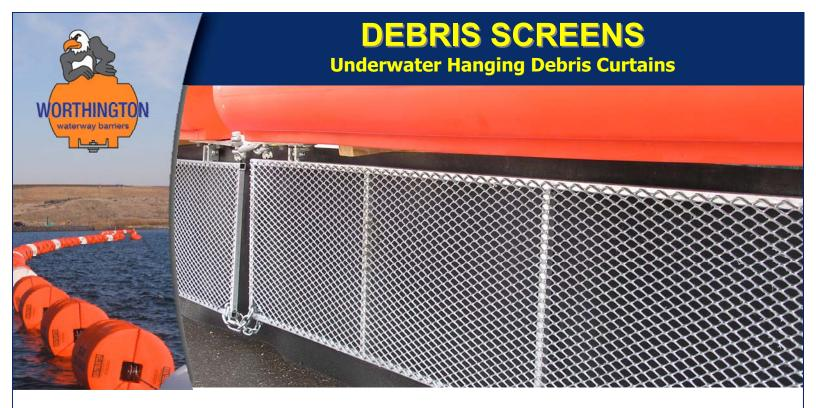
**TUFFBOOM** barriers excel at collecting or diverting surface trash, debris, vegetation and ice. For those locations where the debris is just below the surface or where water currents tend to push debris under the boom line, we offer a simple, effective debris screen that can be attached to new and existing boom lines.
